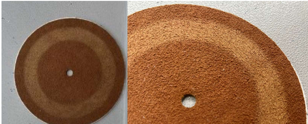
Figure 9. VERA (top left-right) [redacted] after 50 cycles abrasion on TABER® Rotary Platform Abrasion Tester (1000g load of CS-1 Wheel Type).
